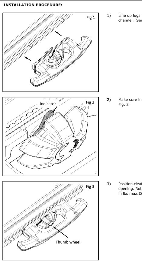
Line up lugs on underside of cleat with notches in the channel. See Fig. 1
