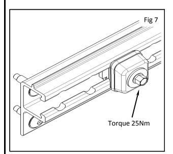
7) Torque bolt to 25Nm using 10mm socket wrench. See Fig. 6
